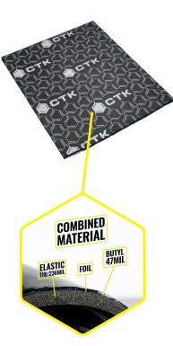
SANDWICH is a combined vibration damping noise and termal insulation material. It consists of a combination of vibration-absorbing material CTK Premium and noise-absorbing material CTK Elastic. It should be used on flat areas of the car floor, doors. It is moisture resistant. The product was created to reduce installation time.
