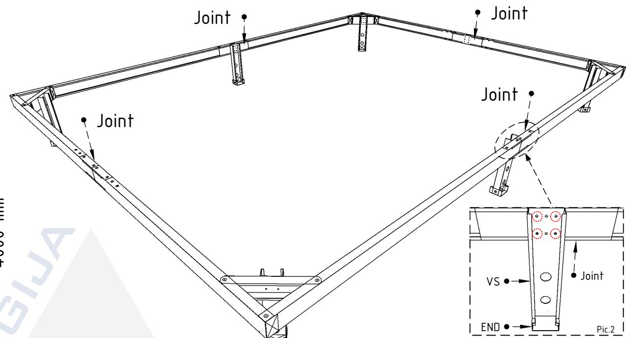
Fix VS element using screws
