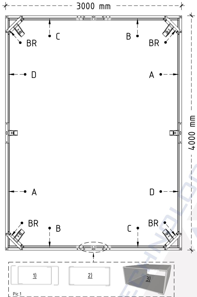
\* Asymmetric profiles allows to make a "box" connection.
