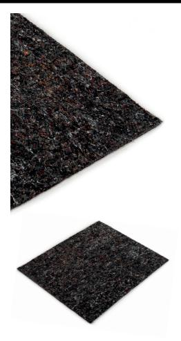
A material made with natural, nonwoven fabric. It provides excellent noiseabsorbing and heat-insulating results. It is very convenient to use and easy to apply on irregular surfaces due to an one adhesive layer on side. CTK Caimat is eco-friendly and wear-resistant.
