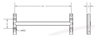
Figure 3-5 Dimensions of bracket
