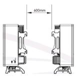
Figure 3-3C Spacing for Back to Back Installation
