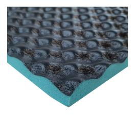
This material is identical to the CTK WaveFix PRO. Its distinctive is a top layer of water-resistant black-colored polyurethane film. Due to the memory effect and wavy shape the material effectively absorbs sound and creates a tight seal between the car body and interior plastic components. Due to its polymer base and moisture-resistant coating and is recommended for use in areas where moisture accumulates.
