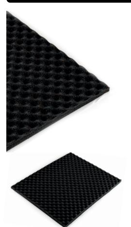
A noise absorbing material based on foamed polyurethane with latex infusion that provides a memory effect. It has an adhesive layer on one side. The undulating soft surface of the material is an effective sound absorber and a seal between the car body and the interior plastic parts. Due to latex infusion, CTK WaveFix is highly durable and non-toxic.
