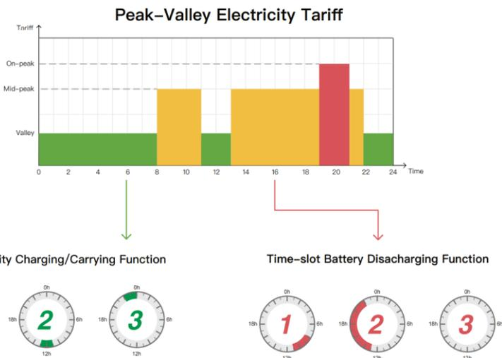
With 3 definable periods, the user can freely set the mains charging/carrying time within the range of 00:00 to 23:59. During the time period set by the user, if PV energy is available, PV energy will be used first, and if PV energy is not available or insufficient, utility energy will be used as a supplement.
