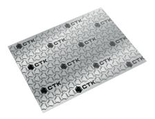
Foilfix is an aluminum foil 200 microns thick with an adhesive layer on one side. It is used for covering holes and openings in body panels as well as the first layer before installing sound dampening materials on the car door frame.
